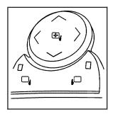
The control on the driver side door operates both outside rearview mirrors.
